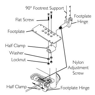
FIGURE 6.9 Installing Adjustable Angle Flip-up Footplates
